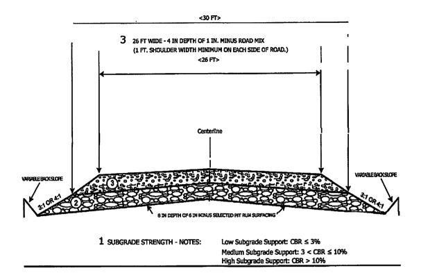
THE SUM OF LAYERS 2 AND 3 MUST ≥ (GREATER THAN OR EQUAL TO) DESIGN VALUES STATED IN ATTACHED TABLE
